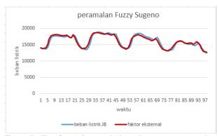
Figure 7. The forecasting result by using temperature and population as external factors
