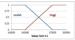
Figure 2. Representation of input variable membership set function.
