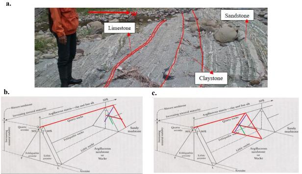
Figure 17. a. The appearance of the CN 19 claystone-sandstone outcrop; b. Placement of claystone composition [8]; c. Placement of sandstone composition [8]
