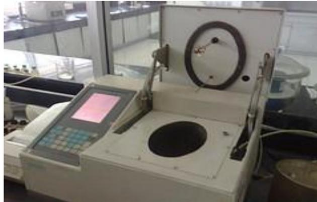
Gambar 1. Bom Kalorimeter
