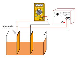
Figure 1. Experimental system of electrocoagulation using Cu electrode
