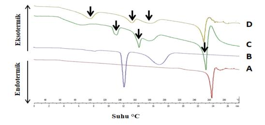
Figure 2. Thermogram of (A) MLX, (B) MA, (C) PM, and (D) Slurry cocrystal
