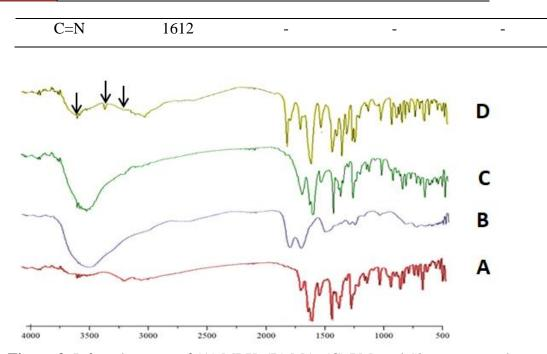
Figure 3. Infrared spectra of (A) MLX, (B) MA, (C) PM, and Slurry cocrystal
