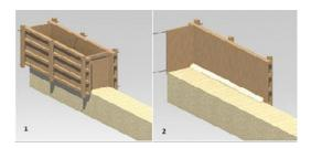
Figure 5. Construction stages of rammed earth wall lift with the face of alterning bricks and lime mortar (Source: Alliche S., 2012)
