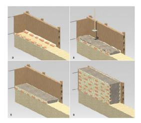
Figure 6. Construction stages of rammed earth wall lift with the face of alterning bricks and lime mortar (Source: Alliche S., 2012)
