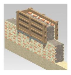
Figure 7. Construction stages of rammed earth wall lift with the face of alterning bricks and lime mortar (Source: Alliche S., 2012)
