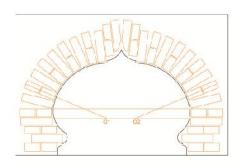
Figure 13. Construction method of Cherchell's arch (Source: Behiri, 2007)
