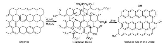
Figure 2. The reactions that occur during the synthesis process of rGO
