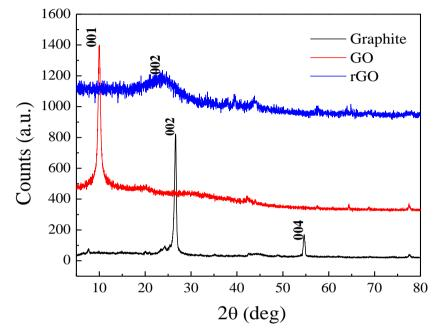
Figure 3. Diffraction patterns from X-rays to samples of graphite, graphene oxide, and reduced graphene oxide
