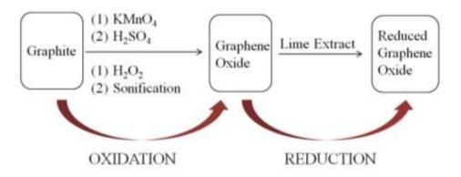
Figure 1. Schema of Reduced graphene oxide synthesis process
