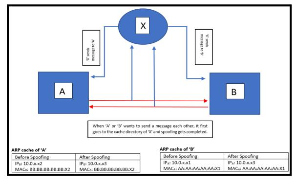
Figure-2: Spoofing method between two clients
