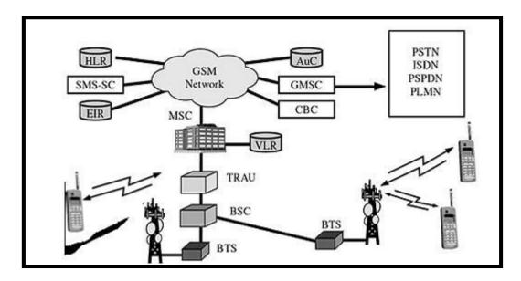
Figure-3: GSM Architecture (J. F. Kurose, 2005 [114])
