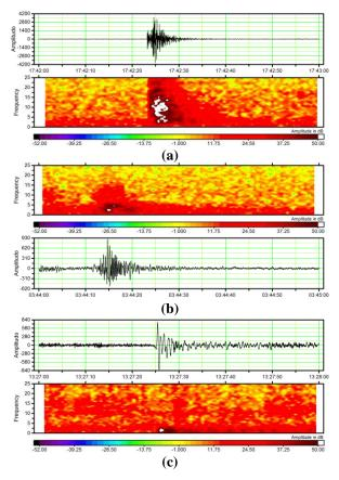
**Figure 4.** Earthquake characters of volcanotectonic on January-November 2015. (a) VT-A earthquake (January 07, 2015; 13:33 WIB), (b) VT-B earthquake (March 03, 2015; 3:44 WIB) and, and (c) LF earthquake (March 19, 2015; 13:27 WIB).
