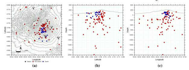
**Figure 5.** The calculation result of hypocenter distribution with GAD method on (a) the contours map of *Gede* volcano, (b) latitude cross section and (c) longitude cross section.
